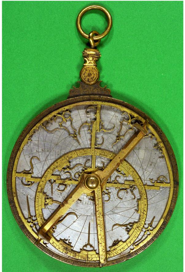
Figure 6: The front of the astrolabe, with a plate, the rete, the alidade (diagonal bar), the rule (vertical bar). The alidade is in principle mounted on the back of the mater
