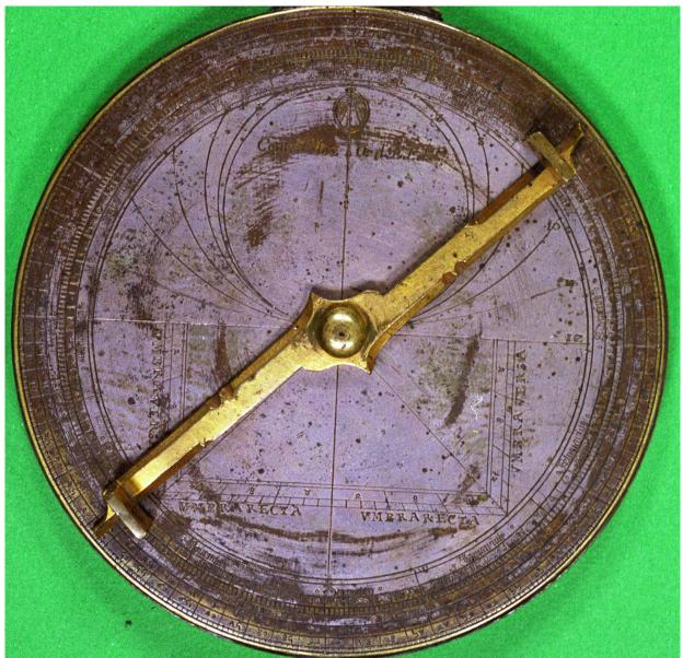
Figure 7: The alidade mounted on the back of the mater
